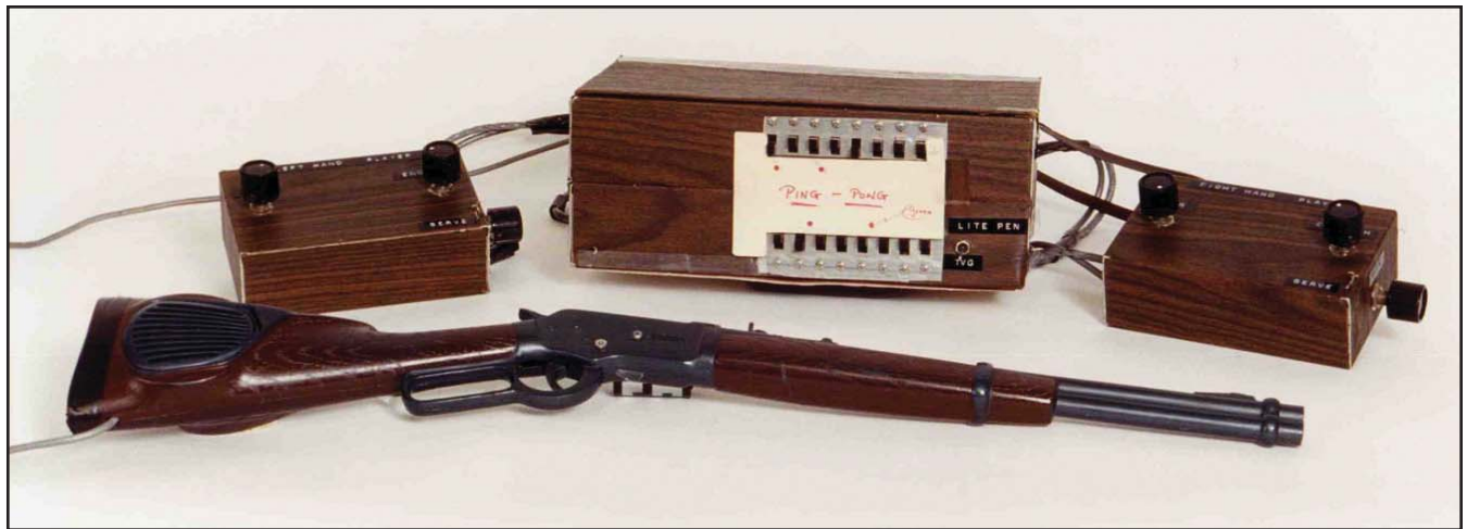
Figure 44 - The Brown Box, our TV Game Unit #7 with its hand controls and gun (1/69)
